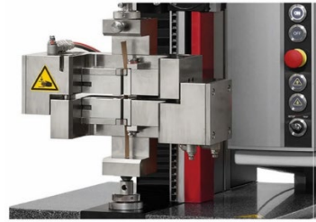
Fig. 12. Short Time Compression Tester. [17]
