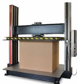
Fig. 8. The compression tester, powered, plate type [15]
