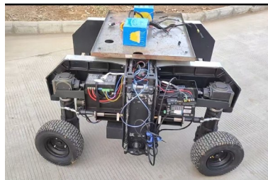
(a) Ackermann steering test
