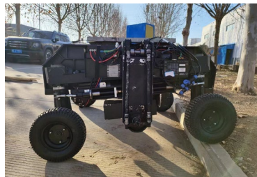
(c) Obstacle-crossing test
