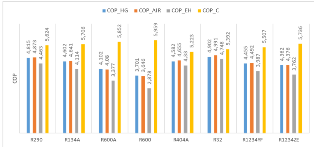
Fig. 10. Comparative COP - Air defrosting, Electric Heating defrosting, Hot gas defrosting, and Cycle COP
