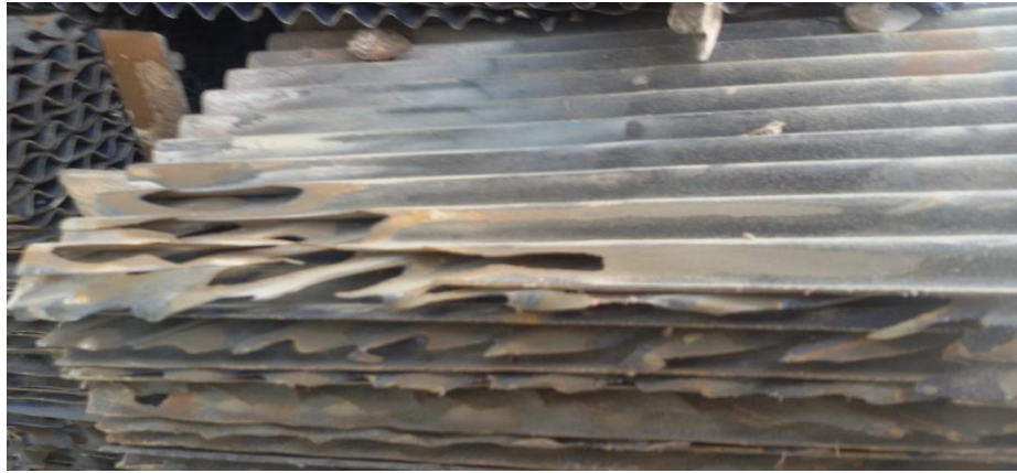
Fig. 4.1. The metal filler of a worn out preheater, formed from the corroded sheet combs
