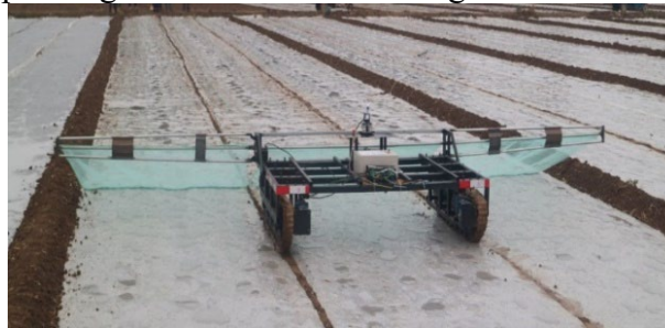
Fig. 9. The actual operation diagram of machine field film breaking.
