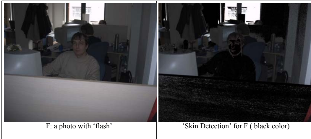
Fig. 1. Typical Skin Detection method: there are many colors with a skin-like chromaticity; for the luminance, we apply two global threshold \rightarrow the far skin regions are not selected due to the inferior threshold.
