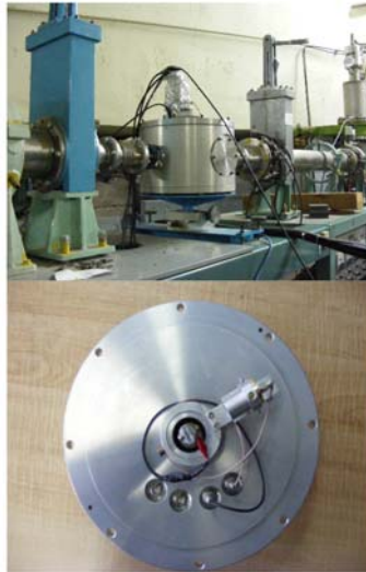
Fig. 2. The scattering chamber mounted on one of the extensions of the Bucharest tandem accelerator (upper part of the figure); the cover of the scattering chamber which contains the stand for the silicon detector and for the sample (lower part of the figure).
