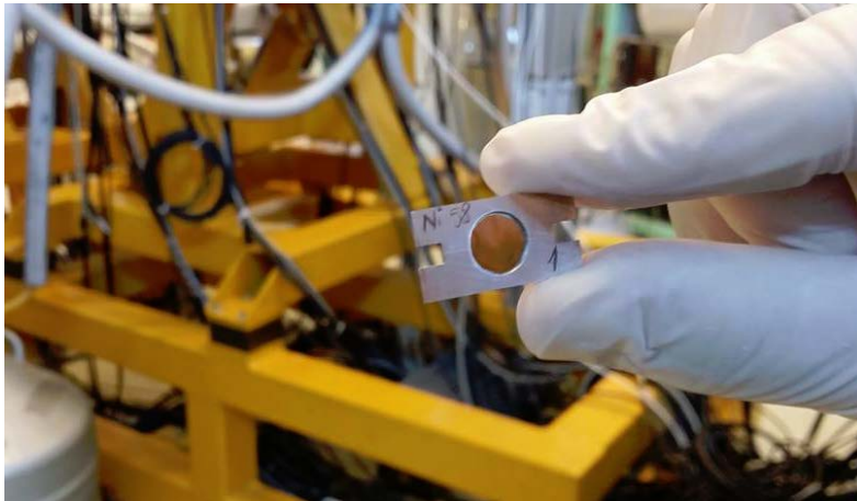
Fig. 1. ^{58}\text{Ni} target produced for the experiment in discussion.
