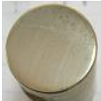
Fig. 2. Sample surface before exposure to cavitation attack
