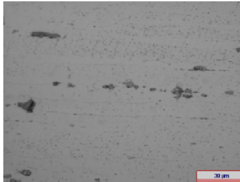
Fig. 6. Sample 3 - Few semicontinuous grain boundary precipitates, 500X
