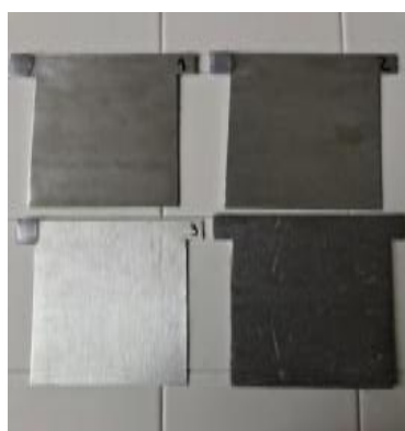
Fig. 1. Aluminum samples and lead cathode used for experiments
