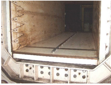
Fig. 4: INCAS Trisonic wind tunnel perforated walls test section
