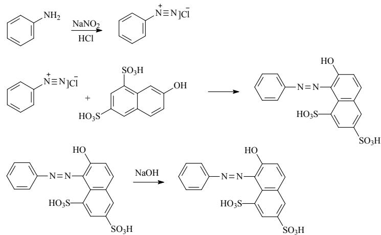
A solution of 5g  $\text{NaNO}_2$  and 25mL water was added, while stirring, over a mixture of 7g (6.8mL) aniline, 37.8g (36mL) HCl 37% and 150mL water. The solution was poured in small amounts, every 10 minutes. To finalize the diazotization process, the stirring continued for another 15 minutes. In this time, the temperature was kept below  $5^\circ\text{C}$ . The resulted diazonium salt was dipped in the following 15 minutes over a solution formed from 17.15g acid G, 6.5g  $\text{NaOH}$
