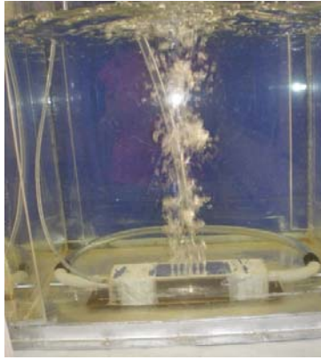
Fig. 11. FBG with 6 orifices \varnothing 0.5 mm in operation
