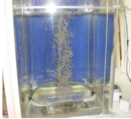
Fig. 9. FBG with 17 orifices Ø 0.3 mm in operation
