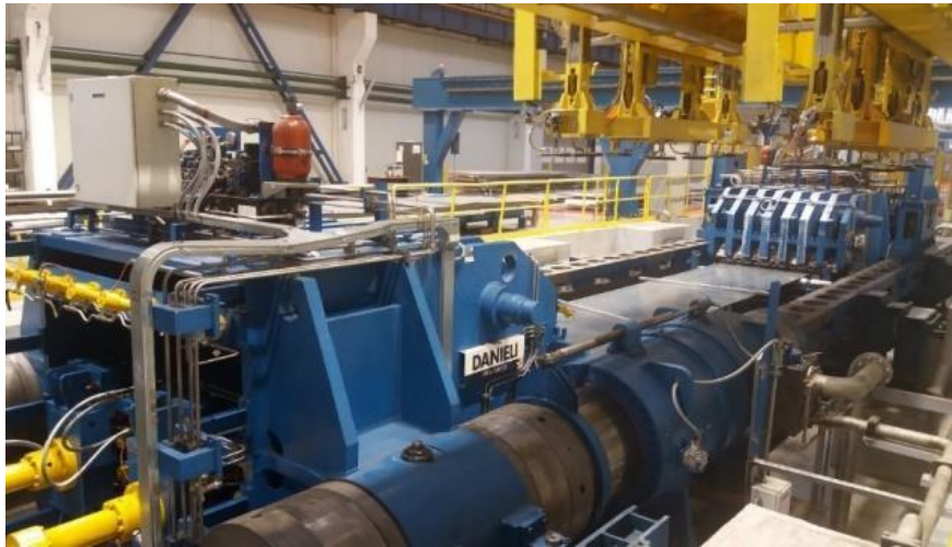
Fig. 1. The independent equipment for the research of the residual stress removal process for the aluminum alloy plates with thicknesses lower than 20 mm.
