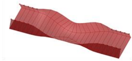
Fig.2. The resulting 3D model with Kangaroo program, using Bending Force.
