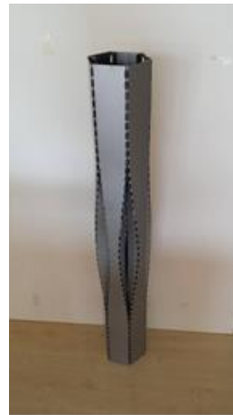
Fig.7. Metallic experimental model (punching with oblong perforations)
