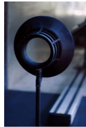
Fig. 3. Casing for small wind turbine at the LAIV research facilities [4].
