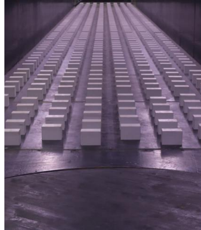
Fig. 6. The variable roughness system of the TASL1-M BLWT.
