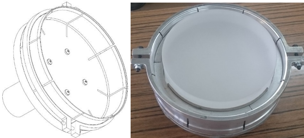
Fig.1. Collet-type chuck (a) 3D model sketch (b) manufactured mechanical part
