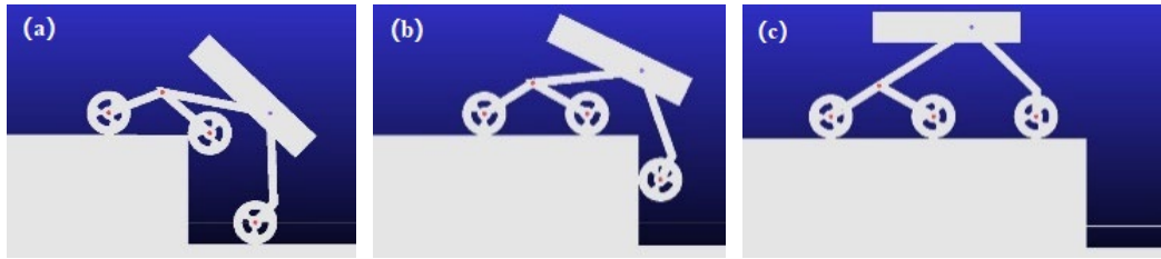
Fig. 7. Obstacle crossing process of the six-wheeled robot: (a) the front wheels are about to climb over the obstacle (b) the front wheels have crossed the obstacle (c) completed climbing the obstacle
