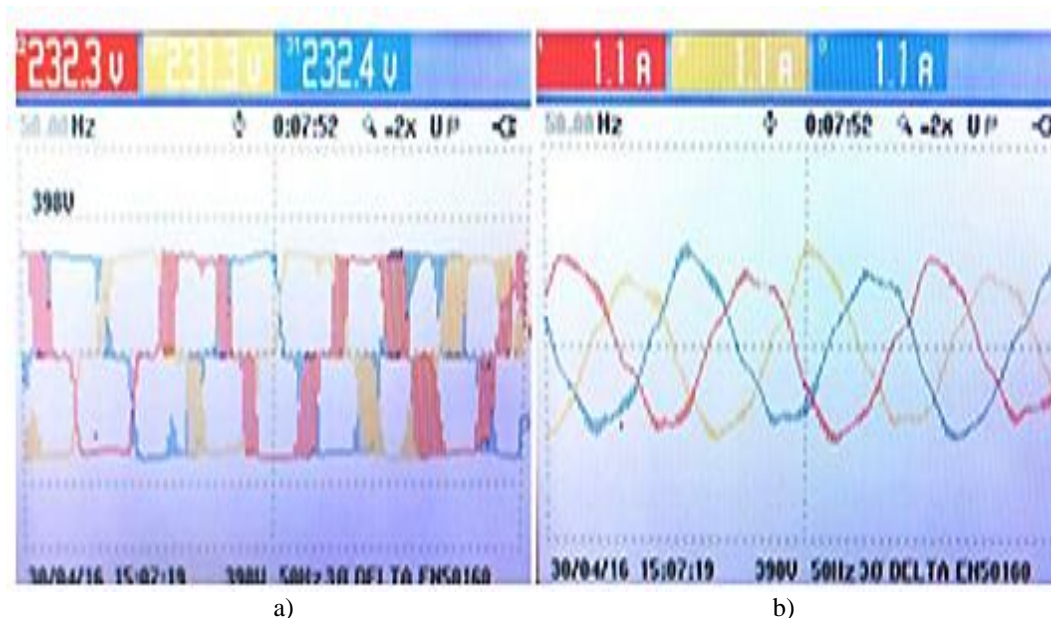
Fig. 11. U (a) and I (b) wave forms at 60 Hz frequency supply at the motor terminals
