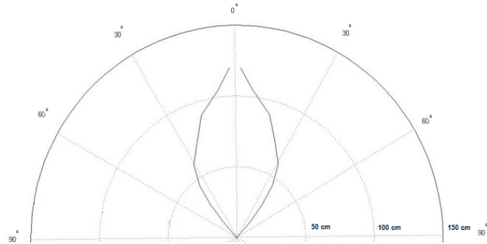
Fig 8. The graphical characteristic of distance-detection angle of the ultrasonic sensors for obstacles located with the surface perpendicular to the detection line of the sensor
