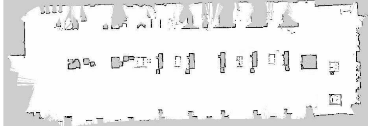
Fig.9. Map created by inspection robot
