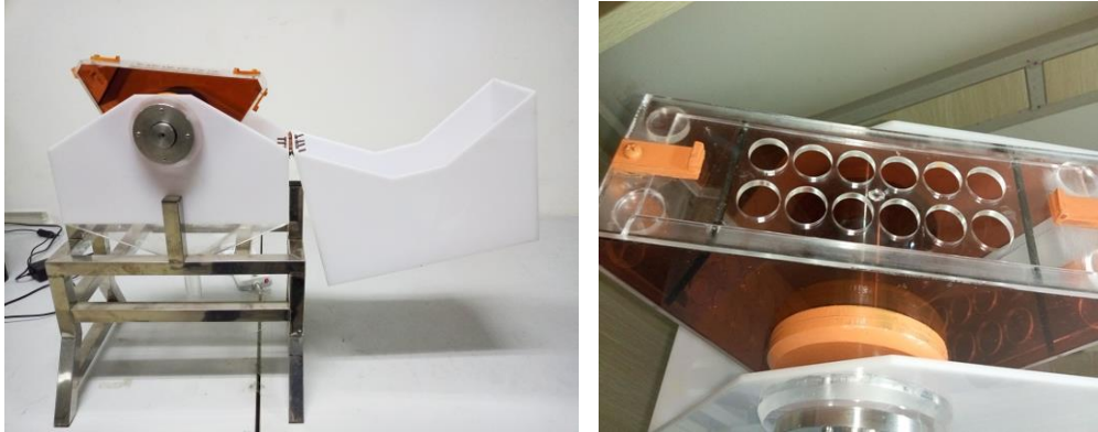
Fig. 11 Physical image of the coins sorting machine
