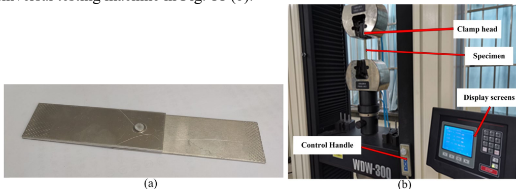
Fig 11 (a) Physical view of the specimen (b) Electro-hydraulic servo universal testing machine The ten static tensile load-displacement curves obtained before and after parameter optimisation are shown in Figure 12.
