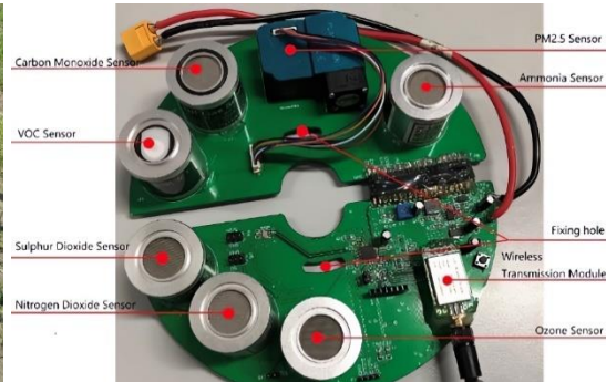
Fig. 3 Six-rotor UAV atmosphere monitoring platform Fig. 4 Picture of UAV-mounted module
