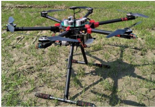
Fig. 3 Six-rotor UAV atmosphere monitoring platform Fig. 4 Picture of UAV-mounted module
