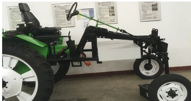
Fig. 1. Vegetable chassis with battery mounted
