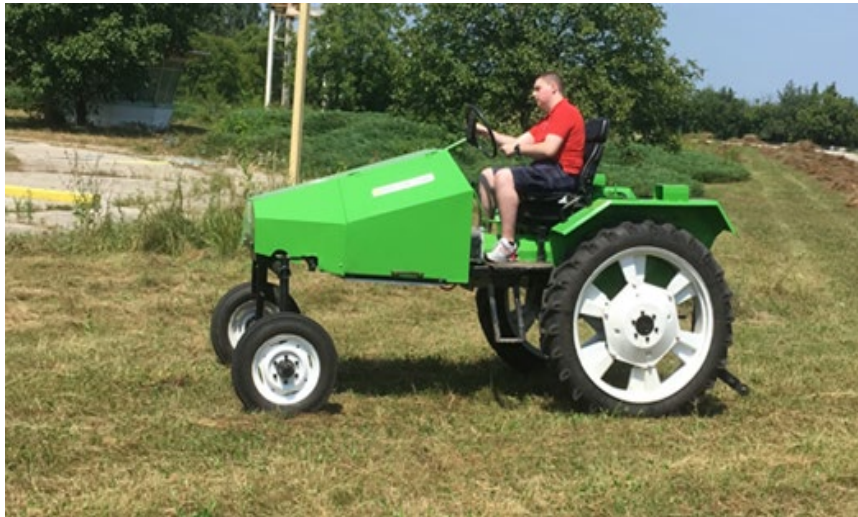
Fig. 3. The electric tractor on the test track within INMA Bucharest
