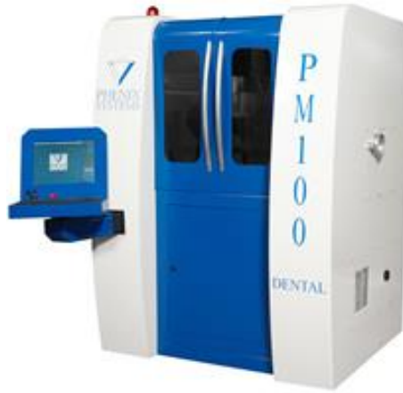
Fig. 1. Selective laser melting machine – PHENIX SYSTEMS PM100 – 200 W.
