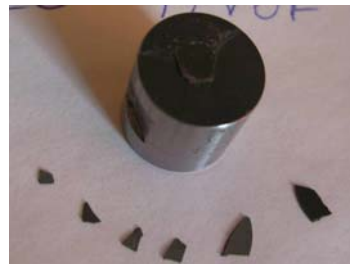
Fig. 3. Thermal sprayed coatings destroyed on direct vibratory tests
