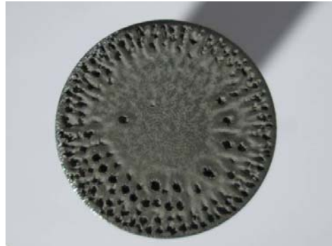
Fig. 5. Sonotrode for indirect vibratory method. Detail on the cavitation eroded surface
