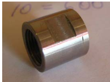
Fig. 2. Sample with cracks on welded overlay
