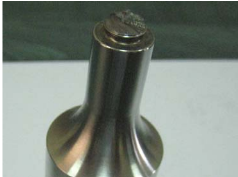
Fig. 4. Sonotrode for direct vibratory method. Detail on the failure area of the thread
