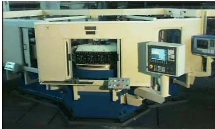
Fig.12. Special machine for boring assembled branch rod
