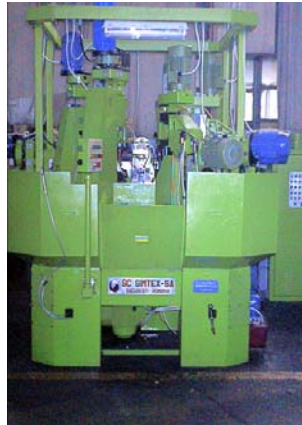
Fig.11. Processing machine for valve body multifactor
