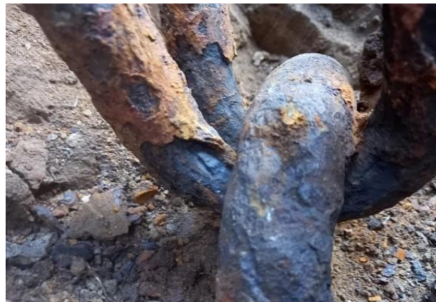
Fig. 7 The underground view of tower B189 anchor connection shows reduced anchor cross-sections, leading to failure during extreme weather and ultimately causing the tower to collapse
