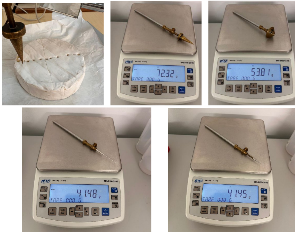
Fig. 3. Aspects regarding the geometric shape and masses of the cones and needles used in the penetration experiments of the analyzed cheese samples
