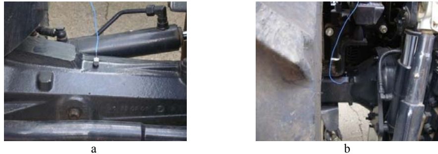
Fig.7. Set-up of the piezoelectric acceleration transducers
