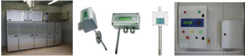
Fig. 3. Dehydrator (left) equipped with an automation and monitoring system (right) and the sensors used (center)
