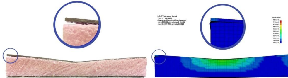
Fig. 8 Delamination between the foam core and the upper facesheet
