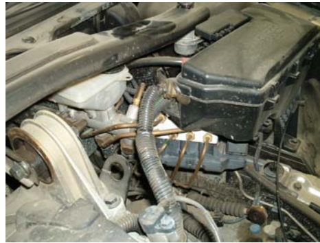
Fig. 2: HCU and ECU location in the engine compartment
