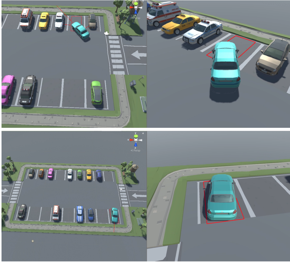
Fig. 3. The agent (blue car) and its environment created in Unity. The left sides are zoomed out versions of the right sides, in which the agent's sensors are visible. In the first set of stills, the agent is in the process of parking on the target spot of the first phase of testing. In the second set, the agent is in the third phase of testing in which the static cars are arranged randomly in the parking lot. This is the spot that the agent has learned best to park on.
