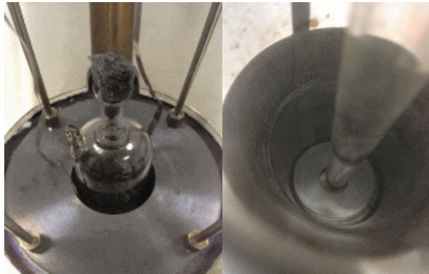
Fig. 1. Fixed point sealed cell that contains pure In
