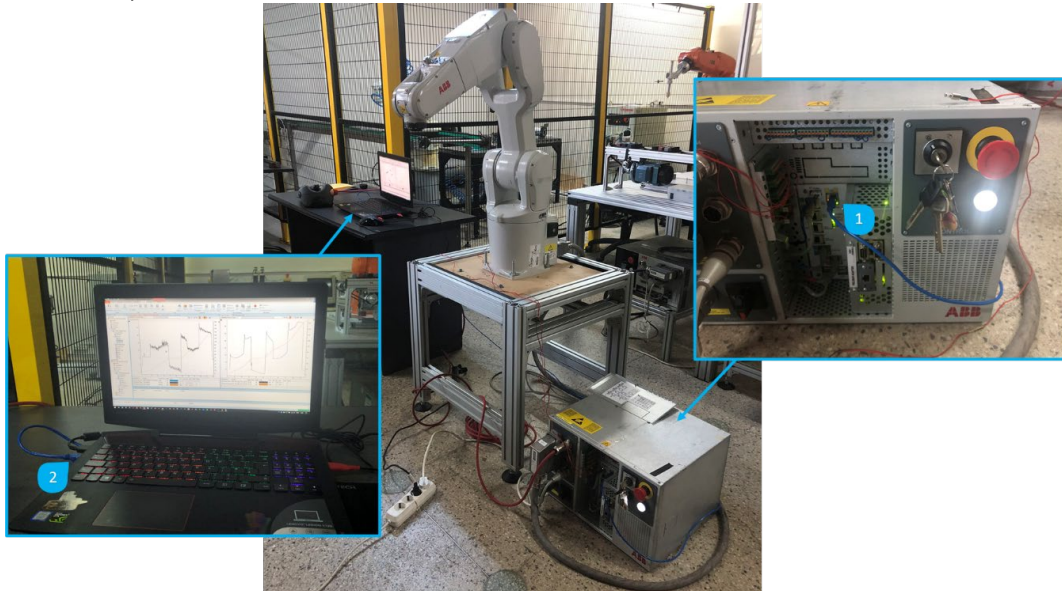
Fig. 9. The experimental setup consisting of an articulated robot IRB 1200, featuring the connection between the IRC5 controller (1) and the laptop running RobotStudio (2)
