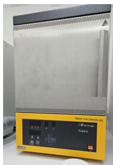
Fig. 2. The sintering furnace (Tabeo-1/M/Zirkon-100, MIHM Vogt) used in the study
