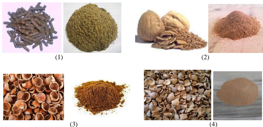
Fig.2. Residual biomass samples: (1)-rapeseed oil cake (raw-left and grinding- right); (2)-walnuts shells (raw-left and grinding-right);(3)-nuts shells(raw-left and grinding-right); (4)-apricot stones(raw-left and grinding-right);
