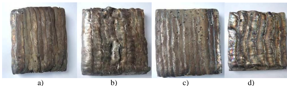
Fig. 1. Samples welded using FCAW process: a) Horizontal (PA) / Sample A1-PA; b) Uphill (PF) / Sample A1-PF; c) (PA) / Sample AC-PA; d) (PF) / Sample AC-PF.
