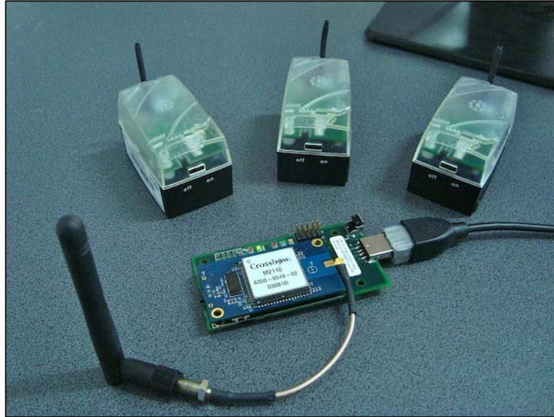
Fig. 2. Memsic IRIS WSN Nodes and USB Radio Base Station
