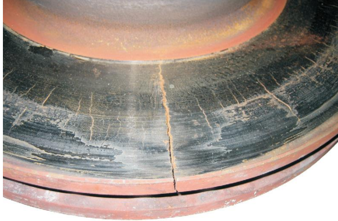
Fig. 1. Crack in brake disc.
