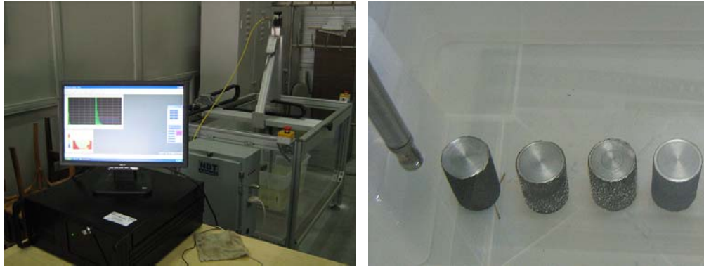
a) b) Fig. 9. a) Experimental set-up; b) OLC 35 samples positioning in the immersion tank.
