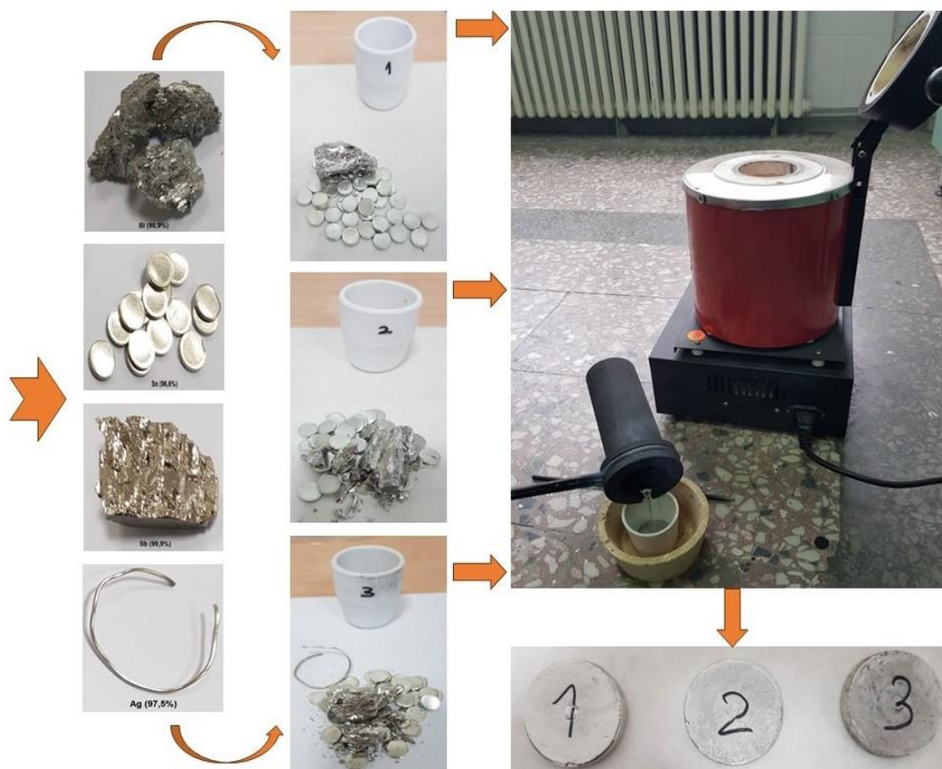
Fig.2. The raw materials used for elaboration, the presentation of the induction furnace and the resulting samples after melting: 1 - Bi60Sn40; 2 - Bi60Sn35Sb5; 3 - Bi60Sn35Ag5
