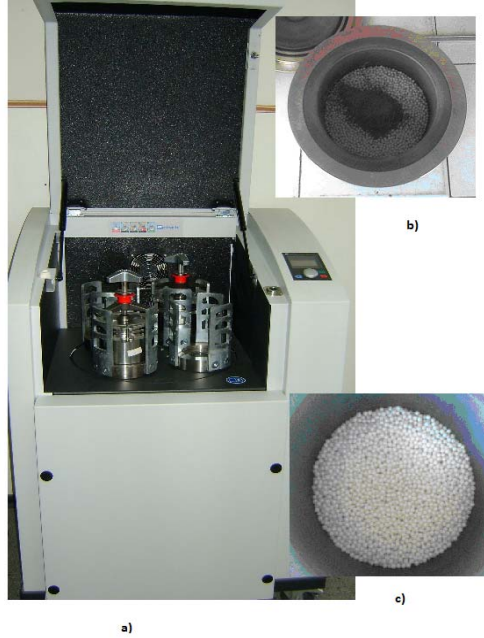
Fig. 1: a) RETSCH Planetary Mill PM 400 and milling chamber, b) milling vial, c) grinding balls
