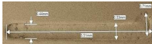
Fig. 13: SEM images of microchannels at 20X on 50 V, duty cycle 82%, tool rotation 400 rpm 19% electrolyte concentration
