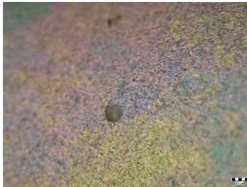
Fig. 6- Macroscopic aspects of the hip rod, with the evidence of a compactity defect on external surface (a,b), and a dimple defect on internal surface (c)
