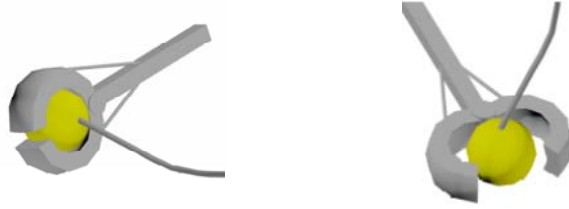
Fig. 9. Basic sensor device holder auxiliary tool designed for simulation
