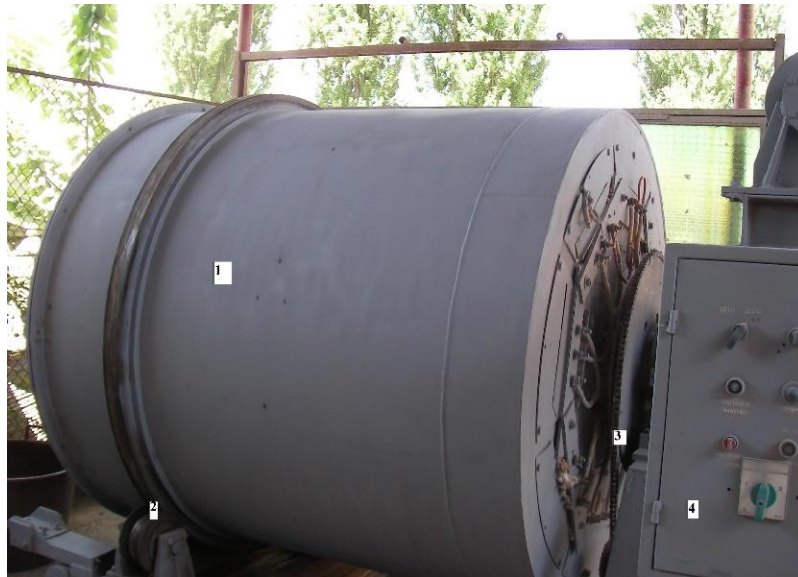
Fig.2 Rotary tubular furnace assembly
